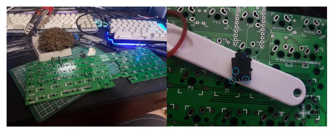
You can opt to use IC sockets as well for the pro micro to enable easy swapping of the pro micro
